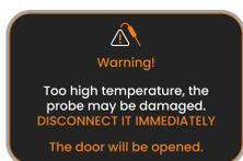
**With the Probe inserted and the Oven cavity temperature above 220°C**, this ALERT pop-up will appear on the display and the oven will automatically open the cooking cavity door. This automatism will remain until the probe is removed or until the temperature inside the cooking cavity drops below 220°C.
